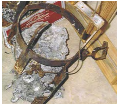
Figure 12.2 Melted propane fuel cylinder after fire in school building
